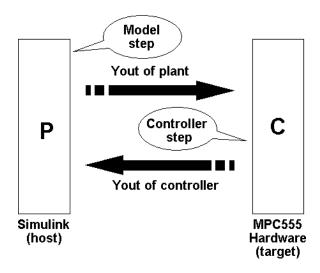
In a PIL simulation, coder product generates efficient code for the control system. This code runs (in simulated time) on a target board using the intended microcontroller. The plant model remains in Simulink without the use of code generation.
