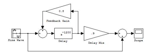
Look for the Delay block in the Discrete library of Simulink and the Gain block in the Commonly Used Blocks library. This model implements an audio signal reverberation scheme. Part of the input audio signal passes directly to the output. A delayed version passes through a feedback loop before reaching the output. The result is an echo, or reverberation, added to the audio output.
