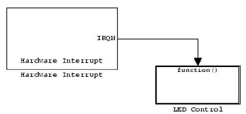
In this model, the C6000 Hardware Interrupt block installs a task that runs when it detects an external interrupt. This task then toggles an external C6416DSK LED on or off.
