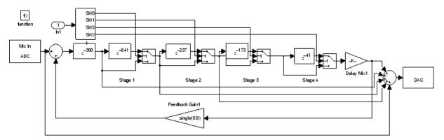
This model also illustrates how synchronous and asynchronous tasks can work together. The code generated for C6416 DSK DIP Switch block runs as a periodic task at the rate of 0.01 s. This is the only periodic task in the model. It runs out of the context of a DSP/BIOS task scheduled via a timer interrupt configured to go off every 0.01 second.
