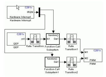
In the preceding figure, the Hardware Interrupt block is set to react on two interrupts. Since only one Hardware Interrupt block is allowed in a model and the output of this block is a vector of length two, you must connect the Hardware Interrupt block to a Demux block to trigger the two function-call subsystems. The function-call subsystems contain the blocks that are executed asynchronously in the context of the hardware interrupt.
