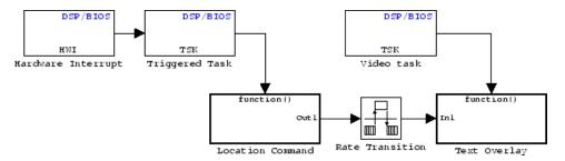
The DSP/BIOS Hardware Interrupt block installs an ISR function that signals a DSP/BIOS task to run when the ISR detects an RTDX interrupt. Signaling between the ISR and DSP/BIOS triggered task occurs via semaphores. This task receives an RTDX message carrying the location command for the downstream Text Insert block in the Text Overlay from the host computer.
