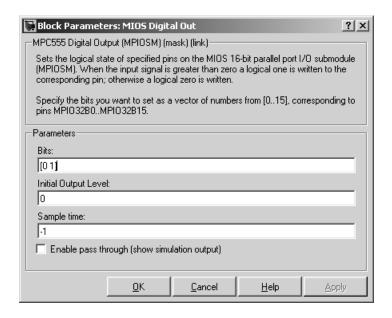
The Bits field is set to the vector [0 1]. The block maps this vector to the MPC555 MIOS digital output pins MPI032B0 and MPI032B1. When the application runs, it will send a pulse signal to these output pins. On the phyCORE-MPC555 board, these signals are connected to two of the LEDs, which will switch on and off at the frequency set in the respective pulse generator blocks.
