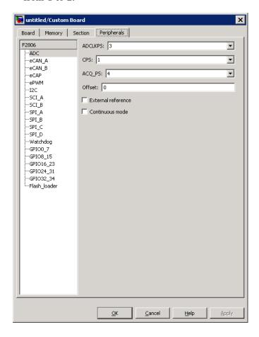
These three prescalers serve to reduce the speed of the clock and to set the acquisition window width. The following diagram shows how these prescalers are used.
