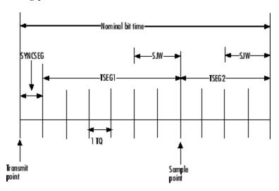
The following illustration shows the relationship between the eCAN bit timing parameters.
