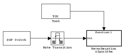
Normally, the algorithms in this type of task run in free-running mode, that is, they run repetitively and indefinitely. However, in this function-call subsystem (shown in detail in the following figure), ADC and DAC blocks suspend the execution of the task until the ADC and DAC data is available.
