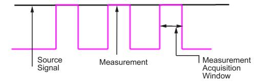
Ideally, as soon as the measurement window is opened, the actual signal coming in would be measured perfectly. In reality the signal does not reach its full magnitude immediately. The measurement process can be modeled by a circuit similar to the one shown in the following figure for the ADC found on the  $F2812\ eZdsp$
