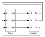
Your starting point in developing a plant/controller system is to model the system as two subsystems in closed-loop simulation. As your design progresses, you can use Simulink external mode with standard targets (such as GRT or ERT) to help you model the control system separately from the plant.
