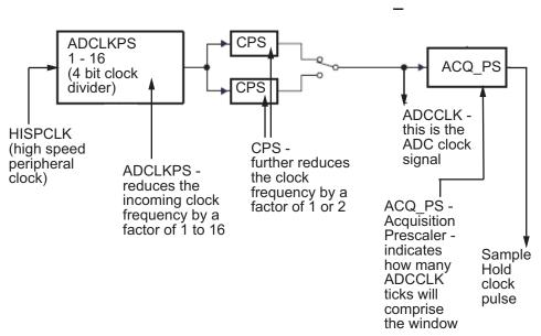
In the preceding diagram, the high speed peripheral clock frequency is received and then divided by the **ADCLKPS**. The reduced clock frequency is then further divided by **CPS**. The resulting frequency is the **ADCCLK** signal. The value of **ACQ\_PS** then determines how many **ADCCLK** ticks comprise one S/H (sample and hold) period, or in other words, the length of the acquisition window.
