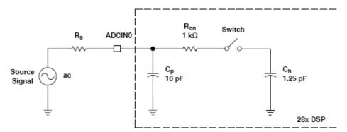
where the measurement circuit is characterized by a certain capacitance. In the preceding figure, when the switch is closed, the measurement begins. In this circuit, which is characterized by its capacitance, the signal received is not in a form of a step function as shown by the ideal measurement, but a ramp up to the true signal magnitude. The following figure shows what happens to the signal when the sampler switch is closed and the signal is received to be measured.
