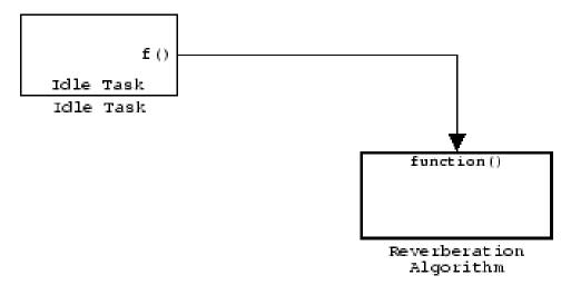
The function generated for this task normally runs in free-running mode—repetitively and indefinitely. However, the ADC and DAC blocks in this subsystem run in blocking mode. As a result, subsystem execution of the reverberation function is the same as the subsystem described for the Free-Running DSP/BIOS Task. It is data driven via a background DMA interrupt-controlled ISR, shown in the following figure.
