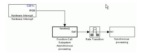
5 The eCAN interrupt on C281x chips is on CPU line 9 and PIE line 5 for module 0. These parameters can be found in the C281x Hardware Interrupt block, C281x Peripheral Interrupt Vector Values figure. Set the hardware interrupt parameters CPU interrupt number(s): to 9, and PIE interrupt number(s): to 5 as shown in the following figure.
