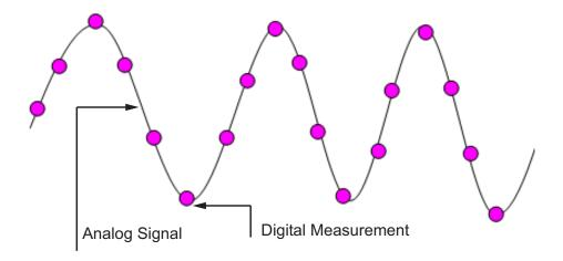
The digital measurement itself is not an instantaneous process, but is a measurement window, where the signal is acquired and measured, as shown in the following figure.
